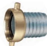
Aluminum Shank with Brass Swivel Nut Female (NPSM Threads)
