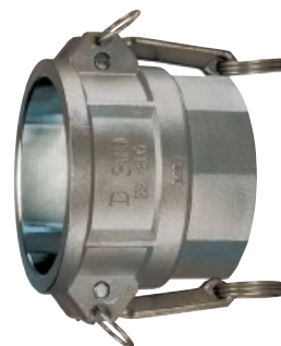
316 Stainless Part D Female Coupler x Female NPT
