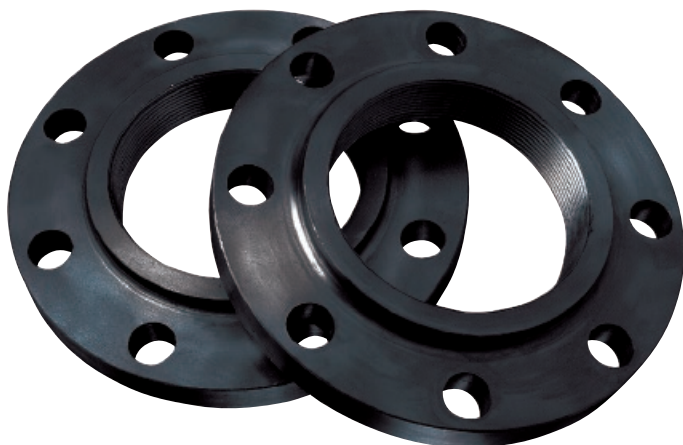
Carbon Steel Forged Raised Face Threaded Flange 150# (ANSI B16.56 & ASTM A-105)
